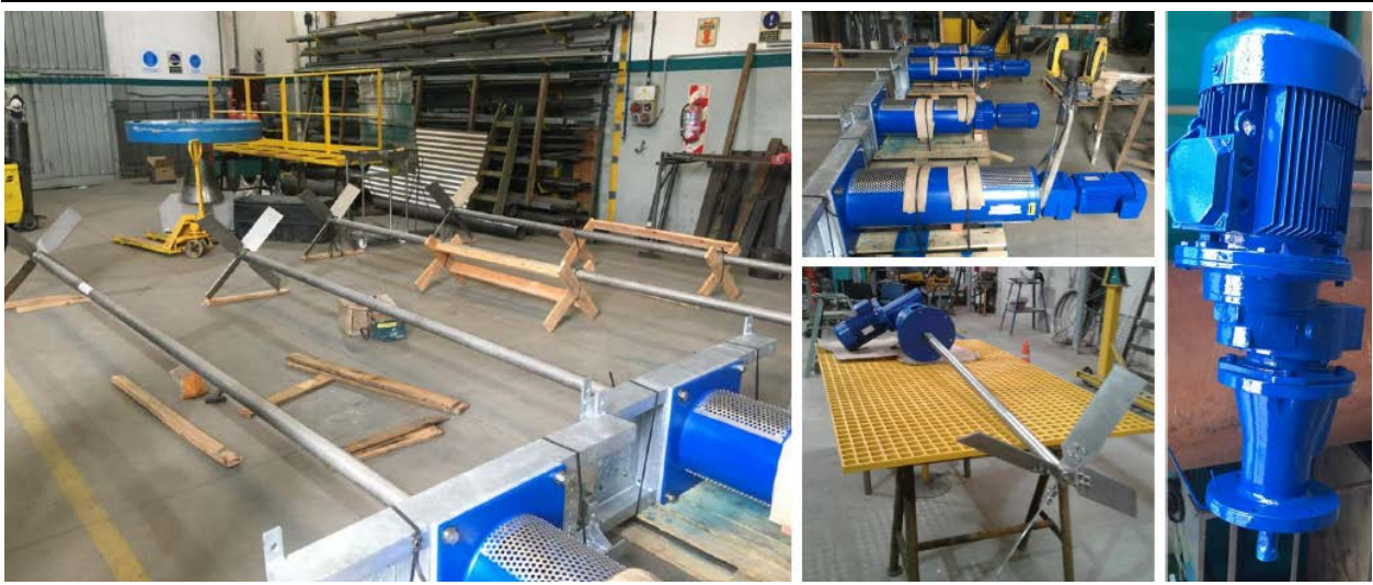
Figure 5. Rincon Lithium Project – 2,000tpa Operational Equipment (Agitators & Motors)
