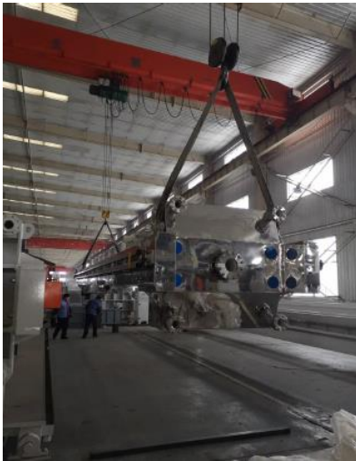
Figures 9-11. Rincon Lithium Project – 2,000tpa Operational Equipment – preparing filters for delivery
