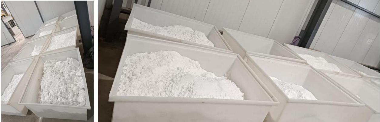
Figures 1-2. Rincon Lithium Project – \text{Li}_2\text{CO}_3 Produced from 2,000tpa Operation Commissioning Works
