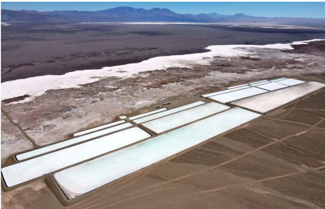
Figure 2. Rincon Lithium Project – 38Ha Operational Evaporation Ponds
